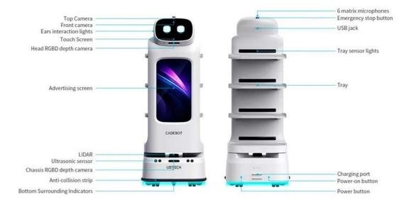
**General Parameters** Overall Machine Dimension: 551\*484\*1265mm Touch Screen Size:
